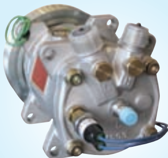
Compressor with LP/ HP switch fitted to high side of rear cap, and low side service port fitted to rear cap.
